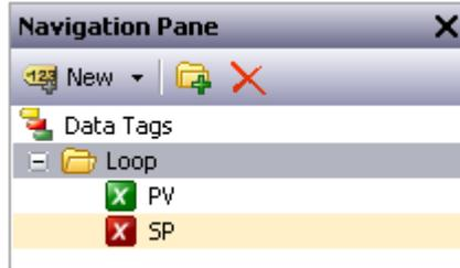
Here, a folder has been created to represent a PID loop, and tags have been created to refer to the loop's process value and setpoint. The tags are referred to in code as `Loop.PV` and `Loop.SP`, using the standard Crimson rules for using nested items.
