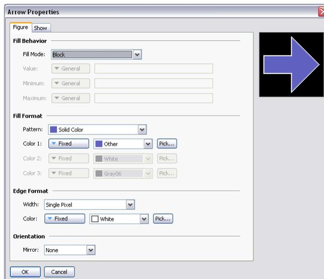
Refer to the previous chapter for details of the standard settings. The *Mirror* property is used to control the direction of the arrow. It is this property that is used to produce the four predefined versions shown in the Resource Pane.
