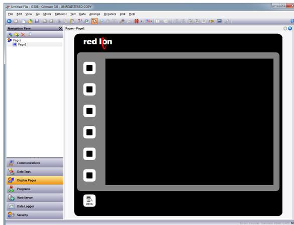
The Editing Pane shows a representing of the target device, including both the keys and the display area itself. At the lowest zoom level, the entire panel will be shown, even if this means allocating less than one pixel on your PC's display for each pixel on the display of the target device. In this situation, pages can still be viewed and most editing can be performed, but accuracy will be somewhat reduced. A warning message to that effect is thus displayed.
