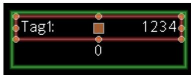
As you can see, the data box is displaying the label from Tag1, indicating that the value of `Data1` that we entered into the data box's Value property is entirely equivalent to the tag to which the data item was subsequently configured. We refer to the process of setting a widget item to a tag as binding that data item to that tag. Binding can be performed in more complex ways, as we shall see later.
