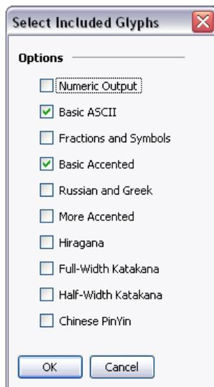
The various options allow specific sets of characters to be included in the font image that is created and downloaded to the target device. Restricting the characters to the ones that are needed for your application will save memory, especially with larger fonts. Note that the Numeric Output option can be used alone to restrict the font to digits, decimal points and those other characters used to render conventional, scientific or hexadecimal numbers.
