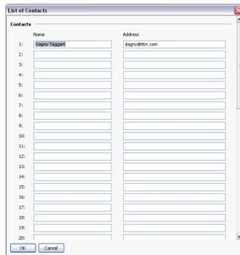
Each entry allows a Display Name and an Address to be entered. The address should be in a format suitable for the required transport. For example, SMTP names should be in the usual name@domain format, while SMS names should be entered as international-format telephone numbers without the leading plus sign. Multiple email addresses can be entered by separating them by semicolons, allowing simple mailing lists to be created.
