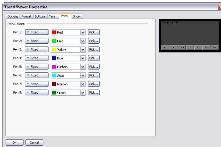
These properties are used to specify eight colors that will be used for drawing the data. The colors are used cyclically, such that a ninth channel will return to the first color. Drawing so many channels is not recommended, as it can produce a very confusing display.
