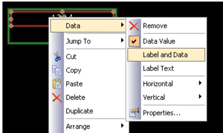
Select the Data submenu, and choose the Label and Data command to configure this data box to display the tag's label as well as its data value. Note the new appearance of the widget...
