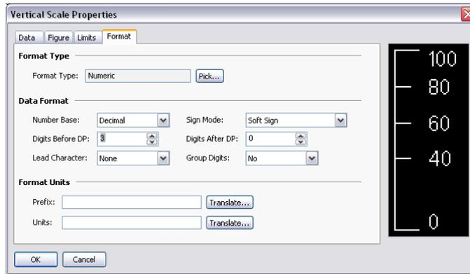
The *Format Type* field specifies the format type to be used when drawing the scale labels. Only general or numeric formats are supported. The selection may not be available if the format is being obtained from a tag. Refer to the section on Using Formats for details of the various other properties that are displayed when a numeric data format is selected.
