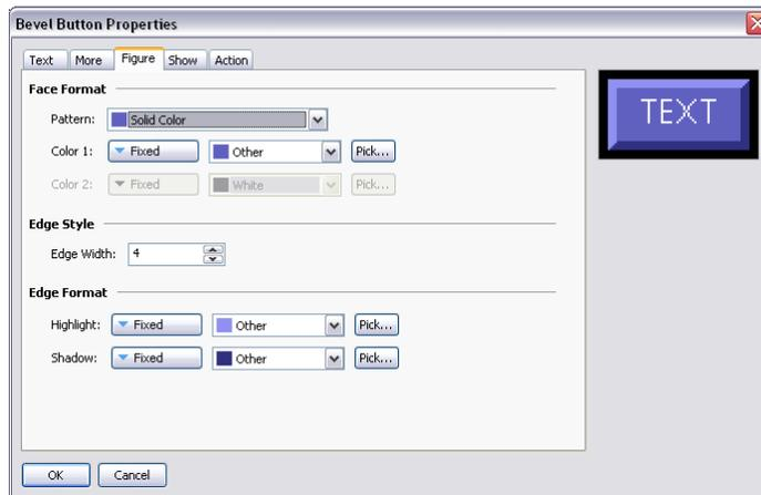
Refer to the previous chapter for details of the standard settings. The *Edge Width* property defines the number of pixels to be allocated to each edge element. Since this primitive always uses an edge style of *Border*, the edge will be sized to twice the defined edge width.
