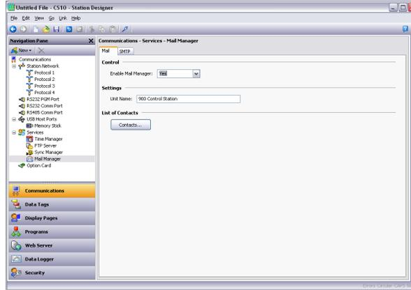
The properties on the Mail tab are used to enable or disable the mail manager, and to provide a name for the device on which Crimson is running. This name will be used within email messages to identify the originator of the message. Applications will typically use the name of the machine to which the device is attached, or the name of the site that it is monitoring.
