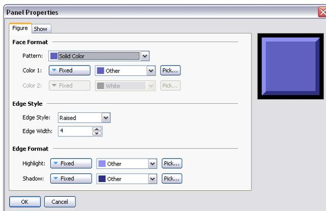
Refer to the previous chapter for details of the standard fill and edge settings. The *Edge Style* selects the type of edge to be drawn, effectively choosing between the three predefined versions shown above. The *Edge Width* property defines the number of pixels to be allocated to each edge element. Primitives with an edge style of Border will have an edge that is sized to twice the defined edge width.
