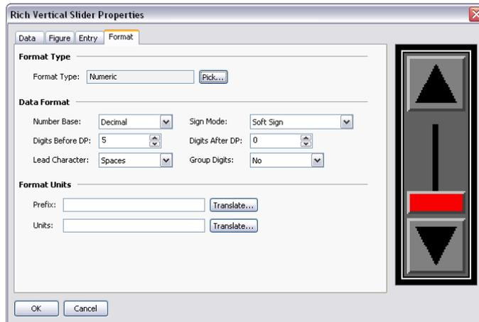
The Format tab defines the data format used by the primitive. Since the primitive doesn't actually display any data, you may wonder why it is needed, and the answer is acceleration: The acceleration of data entry depends on knowing the number base of the data being edited and the position of any decimal point. The other settings are ignored. Note that the format selection may not be available if the format is being obtained from the controlling tag.
