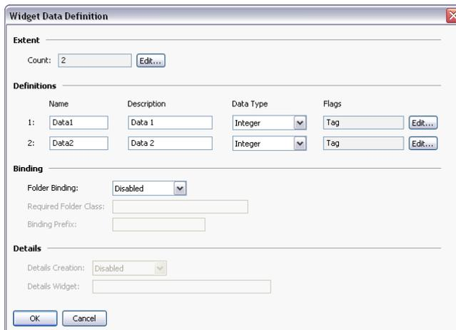
Complete the data fields as shown above, paying particular attention to get the data type right, and to modify the Flags fields to indicate that each data item should be a tag. (The flags field can be edited using the Edit button next to the property.) Press OK to close the dialog box, and note how the widget itself now displays data items in its own properties dialog...
