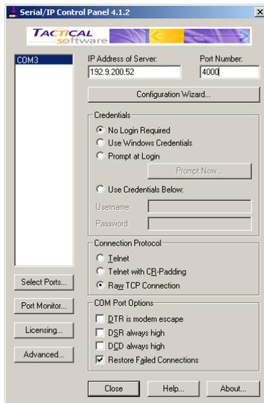
You will now be able to configure any Windows-based software to use the newly-created COM port for download. When the software opens the connection, Crimson will suspend communications on the shared port, and data will be exchanged between the PC software and the remote PLC—just as if they were connected directly! When the port is closed, or if no data is transferred for a minute, communications will be resumed.
