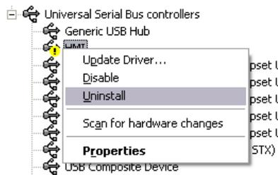
After asking for confirmation, Windows will remove the device from your system. You can now power the Crimson target device off. After a couple of seconds, reapply power and Windows will start the driver installation process once again.
