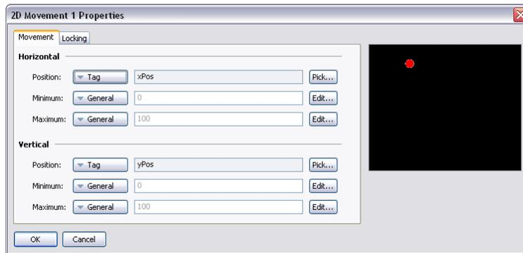
The example above shows the configuration of 2D movement. Polar movement is configured in a similar way. For each dimension of movement, the *Position* value defines where the contents of the group will be placed relative to its outline. The *Minimum* and *Maximum* values represent the limits of the control values. For 2D movement, the minimum settings resulting the group contents being in the top left corner.
