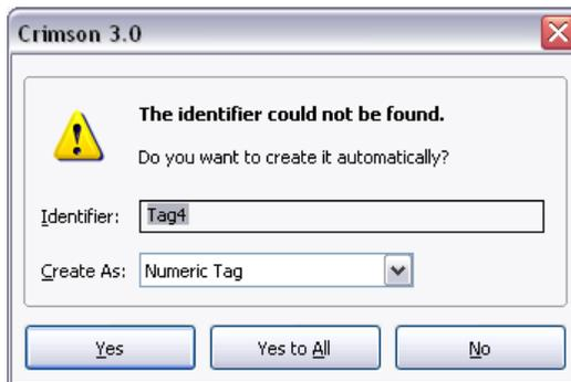
In this example, an expression referencing Tag4 has been entered, but no such tag exists within the database. Crimson spots the error, and asks if you would like to create this tag automatically. The drop-down list can be used to select the type of the new tag, and will contain options appropriate for the context in which the tag was used. The Yes to All button
