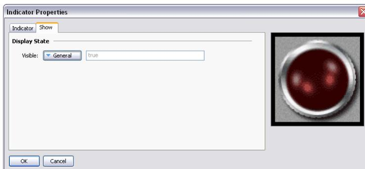
The *Visible* property can be set to an integer expression to show or hide the associated primitive at runtime. A value of zero will hide the primitive, while a non-zero value will allow it to be shown. All primitives are visible by default.
