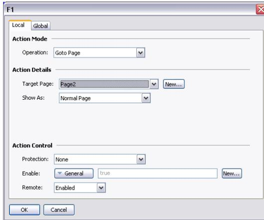
You will notice that this dialog contains two tabs, both of which define an action. The first tab defines the action that will be performed by this key when the current page is displayed, while the second tab defines an action to be performed on every page. These are known as the local and global actions, respectively.
