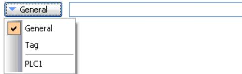
In many situations, you will be configuring these properties to be equal to the value of a tag, or to the contents of a register in a remote communications device. In these cases, you will either be dragging items from the Resource Pane, or you will be clicking the appropriate option on the drop-down menu, and then selecting the item from the resulting dialog box.
