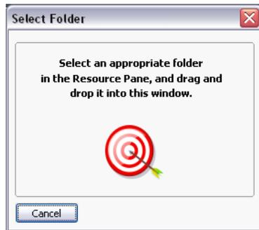
If we drag the Loop folder from the Resource Pane and drop it on the target, the widget's data items will be automatically bound to the corresponding tags in the folder.
