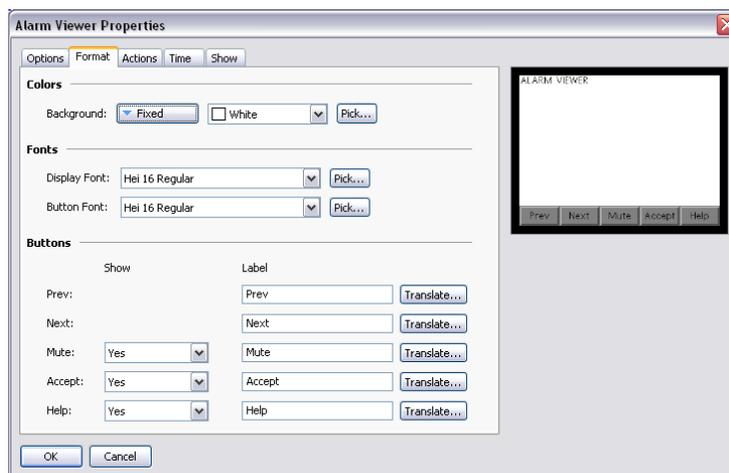
Colors and fonts are specified in the conventional way. The Buttons allows some of buttons at the bottom of the viewer to be disabled, or to allow their labels to be edited or translated for international applications. Remember that translatable strings can be set to expressions, implying that the label on a button can be customized at runtime.
