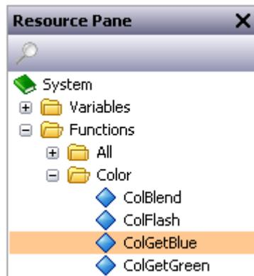
As you can see, variables and functions are grouped into categories. When a function is selected, its return type and argument types are shown on the status bar. Dropping a function into your code enters the appropriate text, and places the text cursor in the parentheses following the function name, thereby allowing you to enter the required arguments.
