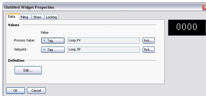
In other words, each data item has been bound to the tag within the selected folder that has a name equal to its own data item name. Think for a second about how powerful this is: You can define multiple properties and bind them in a single operation, reducing design time and allowing better reuse of previously designed items.
