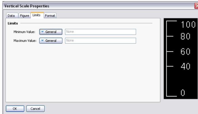
The properties on this page are used to set the minimum and maximum values to be shown by the scale. Expressions may be specified, in which case Crimson will dynamically update the scale at runtime, choosing tick marks and label positions appropriate to the new values. These settings may not be available if a tag has been chosen as the source of the limit values.
