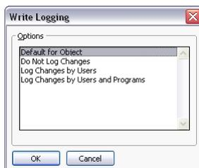
The selection indicates whether changes made to a tag by users or by programs should be logged. This facility allows you to create an audit trail of changes to your system, thereby
