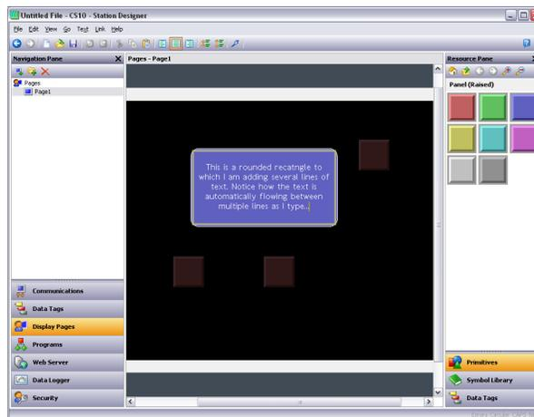
Note first of all how the bounding rectangle for the primitive is shown in yellow, and how all the other primitives on the page are faded out. Note also how the text editor automatically splits the text across lines. Try resizing a primitive containing text, and you will see how Crimson reflores the text to fit into the new shape.
