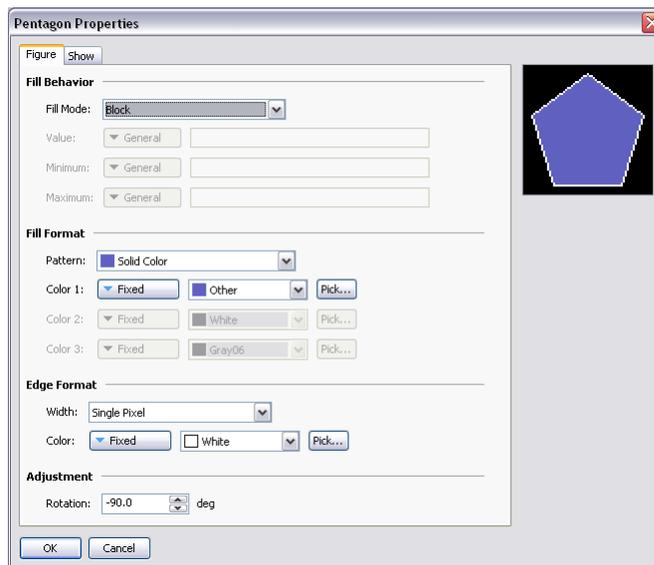
Refer to the previous chapter for details of the standard fill and edge settings. The *Rotation* property can be used to rotate the polygon within the bounding rectangle. The x- and y-axes are scaled such that the overall width and height of the polygon fill the rectangle.
