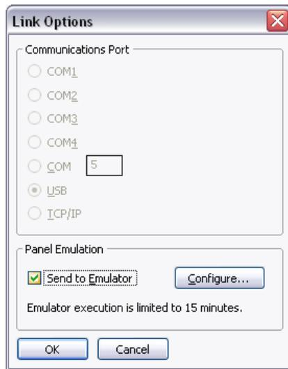
Its enable state may also be toggled using the Emulator button on the toolbar...
