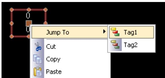
Select `Tag1` to jump to that tag, and enter a value of 1234 in the Simulate As property. Use the **ALT+LEFT** key combination or the Back button on the toolbar, and note how the widget is continuing to track the tag data...
