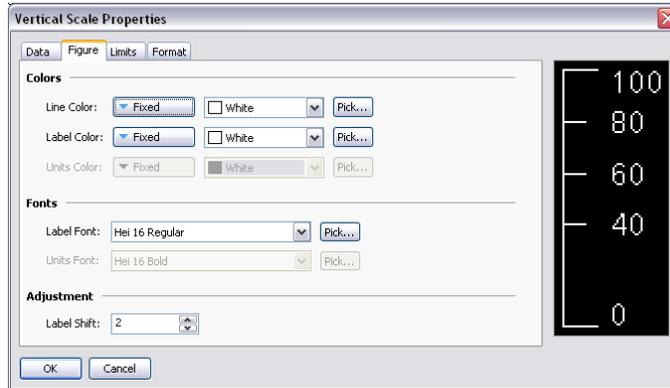
The properties on this page define the colors and fonts used for the scale. Refer to the previous chapter for details of the standard properties. The *Label Shift* property can be used to move the labels up or down relative to the tick marks, producing more attractive results when working with fonts with spacing above or below the character glyphs.
