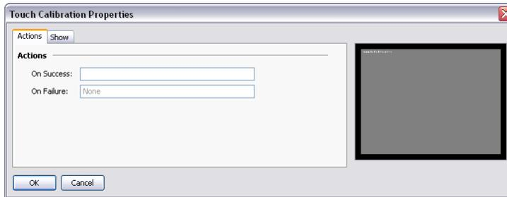
Its primitive-specific properties define the actions to be taken when calibration has either succeeded or failed. These properties are typically configured to return to a menu screen or to otherwise move away from the calibration page.
